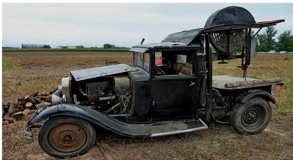
An Opel Kapitän built in 1939, converted in the 1940s to wood gas propulsion and a Citroen V4A built in 1930, converted in 1950 into a mobile band saw.
